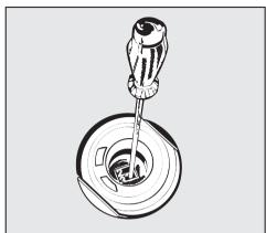
The dosage adjuster in the opening has settings adjustable from 1 to 6 (1-6 ml). It is preset to "5" (10 ml) as the recommended dosage for **neutralizer**.
